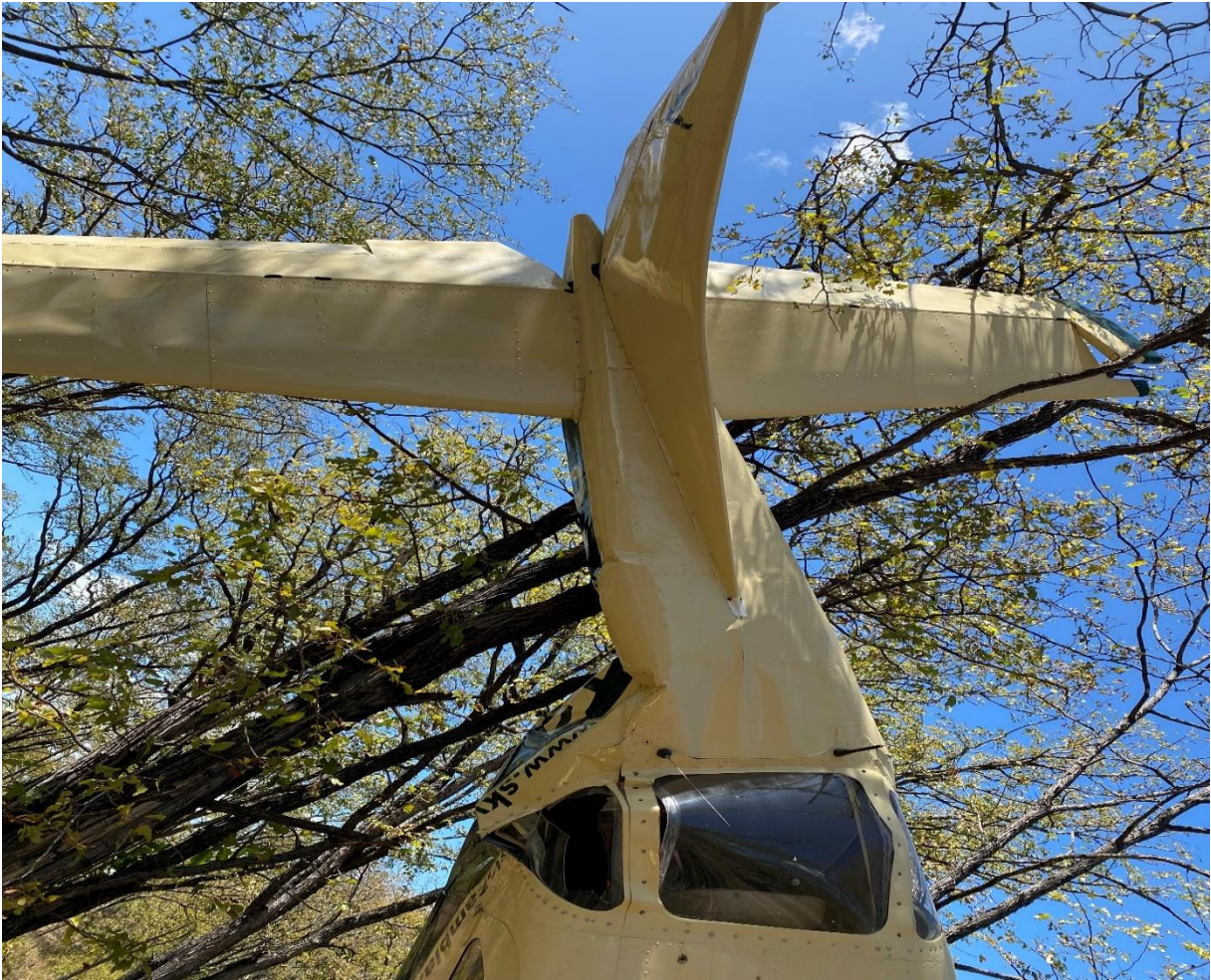
Fig.6: Tail Section Bent and Damaged
