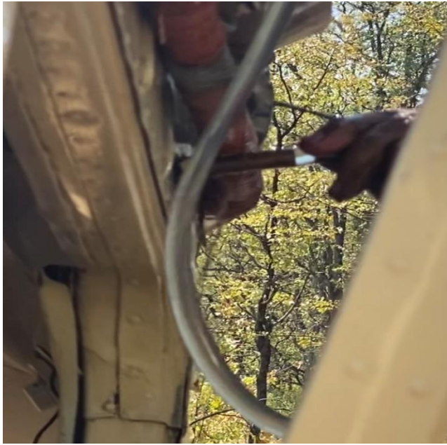
Fig.12: Fuel Being Fed Directly Into the Left Side Fuel Inlet On the Aircraft Fuselage
