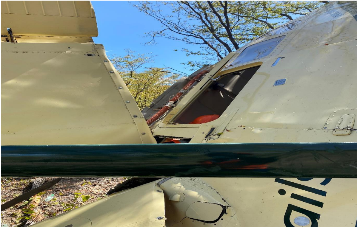
Fig.4b: Left Wing Partially Detached from Aircraft Fuselage
