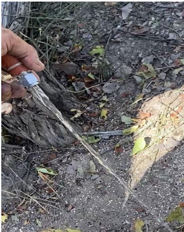
Fig.14: Fuel from the Right Fuel Tank Exiting at the Engine Outlet
