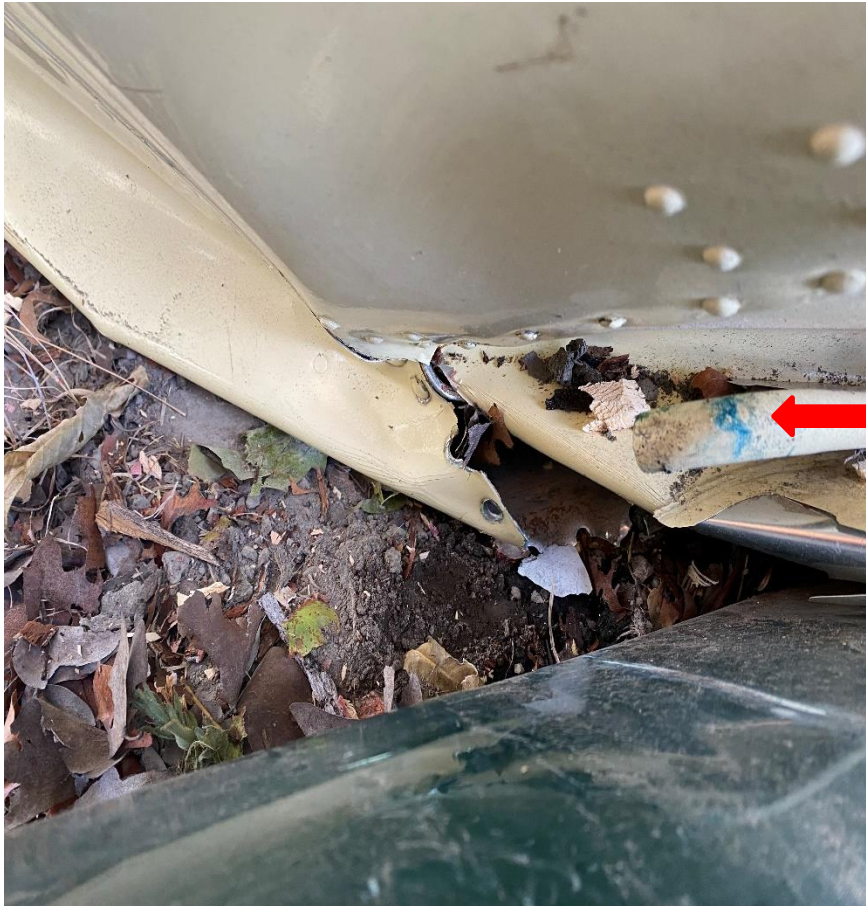
Fig. 15: When fuel is in contact with the aircraft fuselage, decolourisation occurs as seen in the photo. This decolourisation occurred when the team was conducting on-site investigations.
