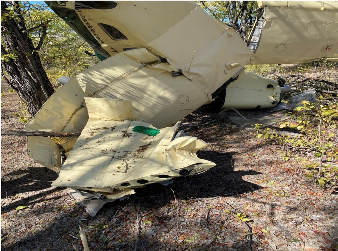
Fig.3: Right Wing Damaged and Folded
