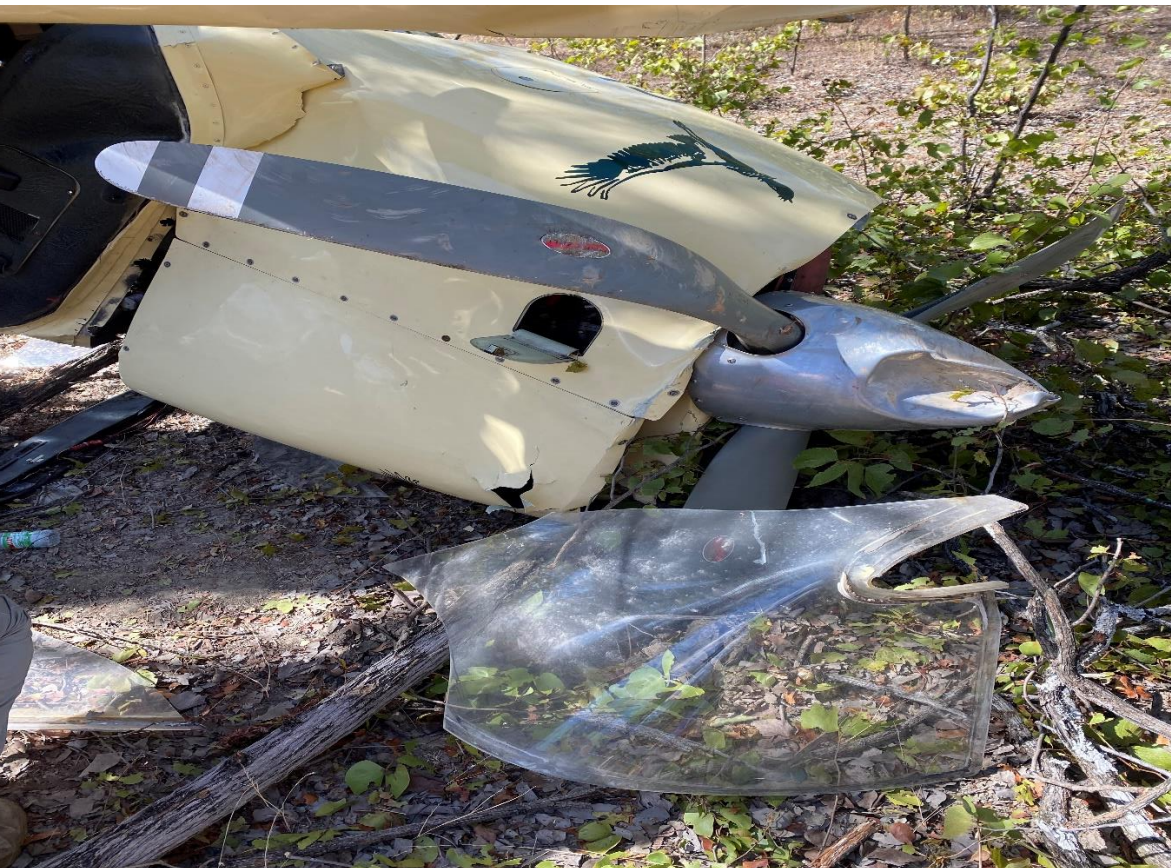
Fig.2: Propeller Damaged with One Propeller Blade Bent Backwards and Broken Windshield Pieces
