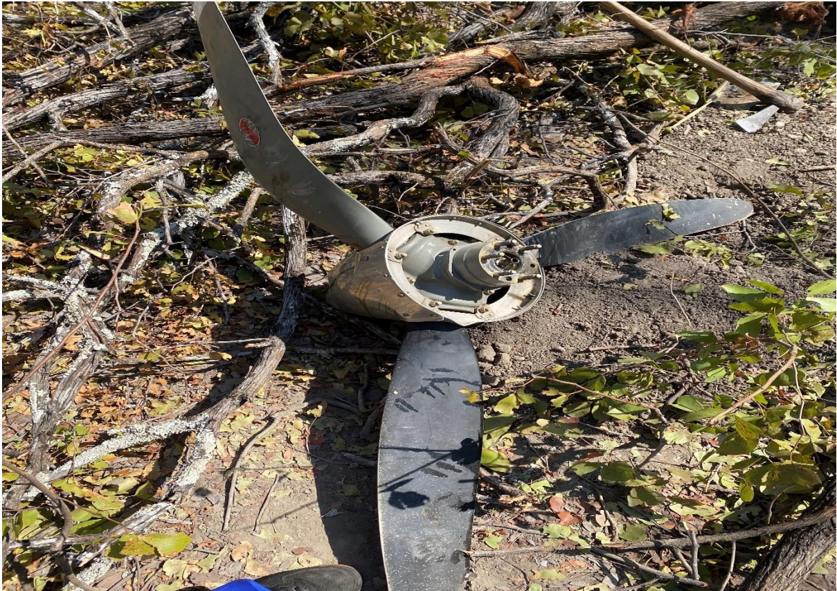
Fig.8: Propeller with One Propeller Blade Bent
