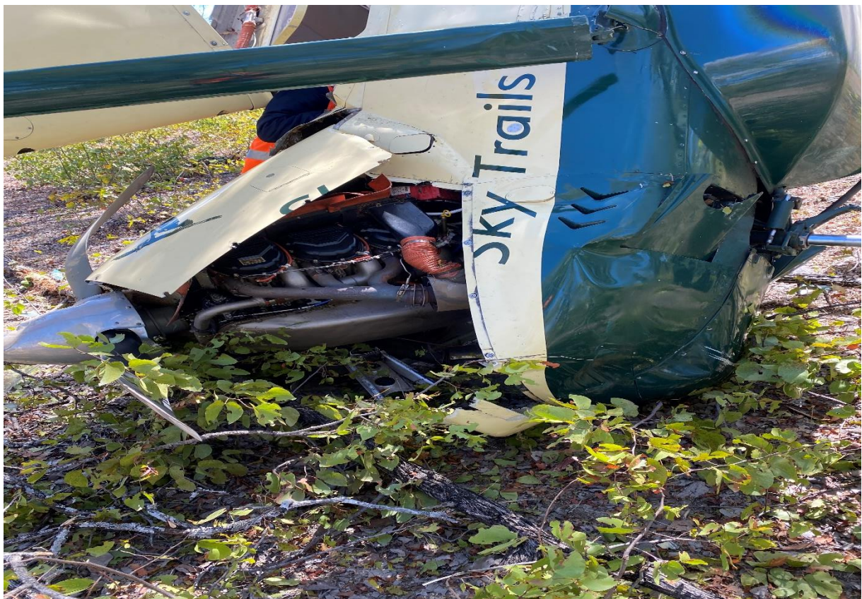
Fig. 5: Engine Cowlings Damaged and Unmounted
