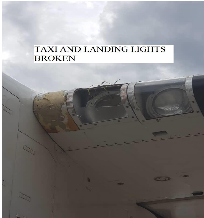
Fig.7 Taxi and Landing Lights
